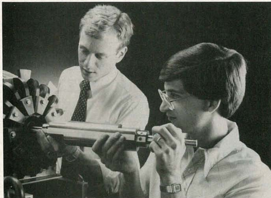
REM TECHNOLOGIES' VICE-PRESIDENT OF ENGINEERING, Jim Grant (l.), and technician John Cestra, are shown inserting a rotor machined from a single piece of steel into the Homopolar Inductor Drive (HiDrive) motor. That rotor is the only moving part of the HiDrive motor.
