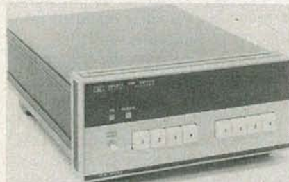
FIG. 10—THE HP 59307A DUAL VHF switch module provides two 1P4T switches controllable by the GPIB.
