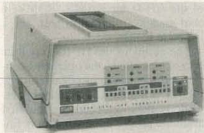
FIG. 14—THE FLUKE 1120A IEEE-488 translator can up-grade an instrument not specifically designed for the GPIB.
