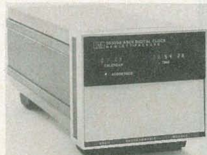
FIG. 11—THE HP 59309A GPIB digital clock displays month, day, hour, minute, and second, and upon command will output time via the interface bus.
