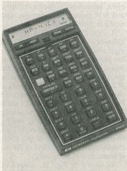
FIG. 15—THE HP-41 IS A combination handheld calculator and controller for the HP-IL.
