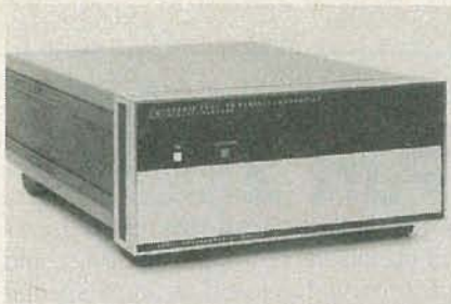
FIG. 7—THE HP 59301A ASCII-to-parallel converter accepts byte-serial ASCII characters from the GPIB, then converts them to parallel output.
